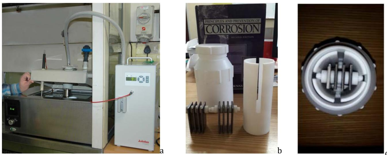
**Figure 1:** Experimental setup: (a) water bath with immersion cooler setup, (b) corrosion reactor components: Teflon bottle, cylindrical corrosion rack and steel coupons, and (c) complete assembly for safely simulating the corrosive conditions in HF.
