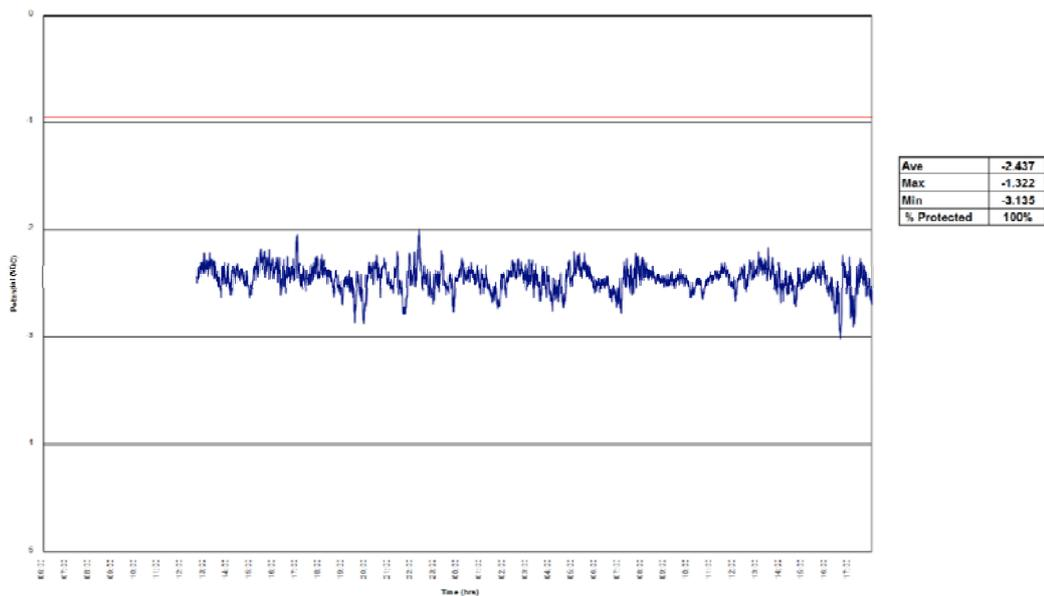
**Fig 3: The graph illustrates full protection in terms of the  $-0.95V$   $Cu/CuSO_4$  "ON" potential and % time protected criteria**
