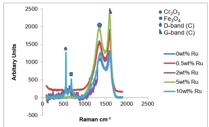
**Figure 6: Raman Spectra for the smooth surfaces on the samples after exposure.**
